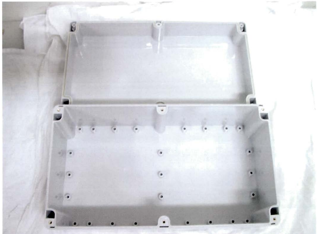
There is no trace of water inside.
