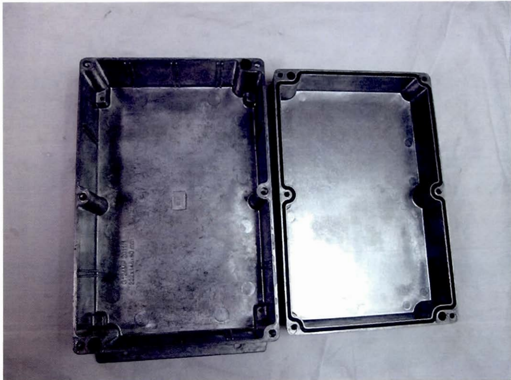
There is no trace of water inside.
