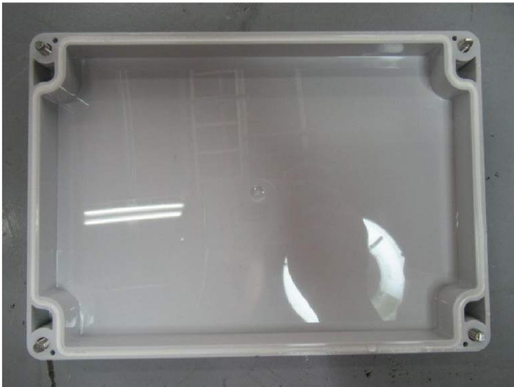
There is no trace of water inside.
