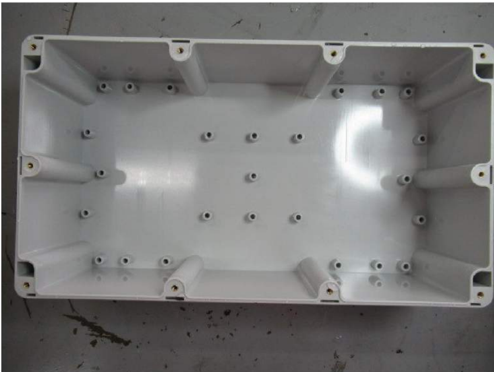
There is no trace of water inside.
